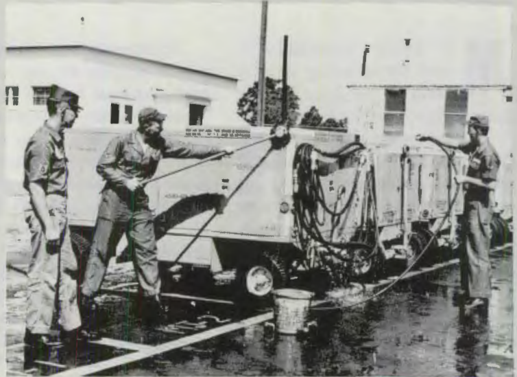
Hydraulic units get their daily washing. This does much to reduce system contamination.
